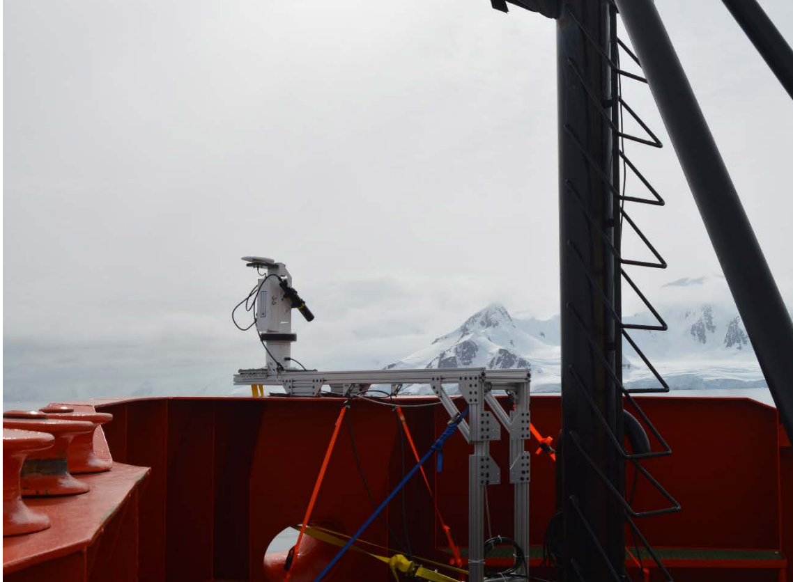
Figure 9: HyperSAS Radiometer on bow of LMG.
